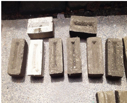
Figure 3. Frogged fabricating rig bricks with & without abaca fibers
